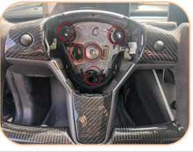
10. Then install the steering wheel, screw in the screw and plug in the steering wheel plug, and then fasten the speaker harness buckle.
