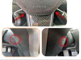
3. There is a hole on the left and right sides of the steering wheel. Insert and Jack the airbag spring with a flat head screwdriver respectively.
