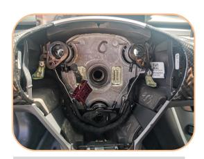
8. Then pull out the steering wheel. If the steering wheel is too tight, shake it left and right and pull it out slowly.
