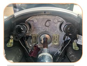
7. Screw out the steering wheel screw with a large H10 wrench.
