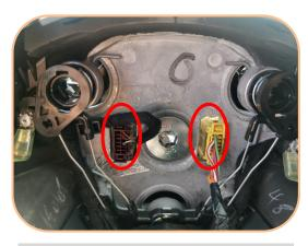
5. Take out the airbag and pull out the airbag plug and steering wheel plug.
