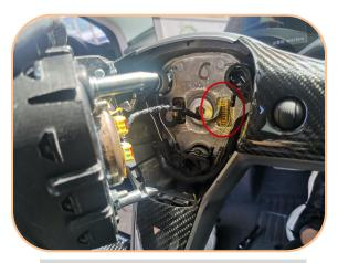
11. Finally, insert the airbag plug, and insert the airbag into the spring bayonet.
