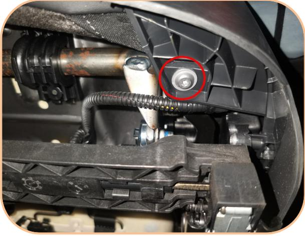
19. Remove a screw on the right side of the bottom of the seat
