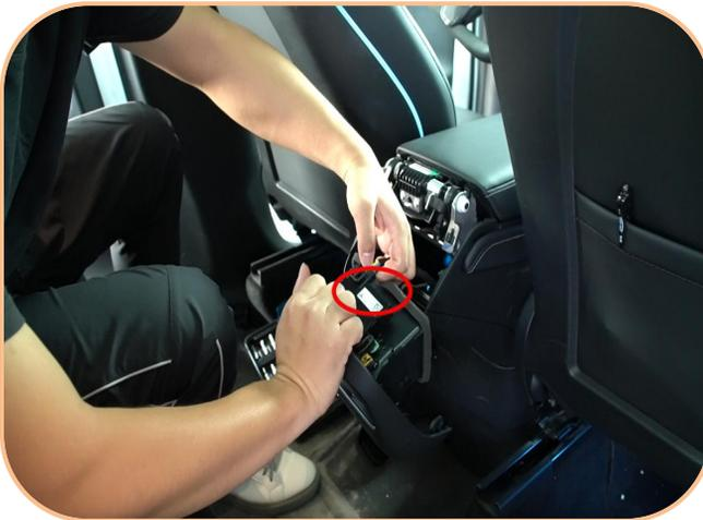
3. Pull off the A/C outlet module plug
