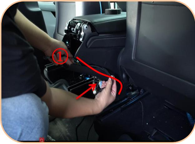
13. Pull harness with **plug ①** to the upper part and restore the cover plate
