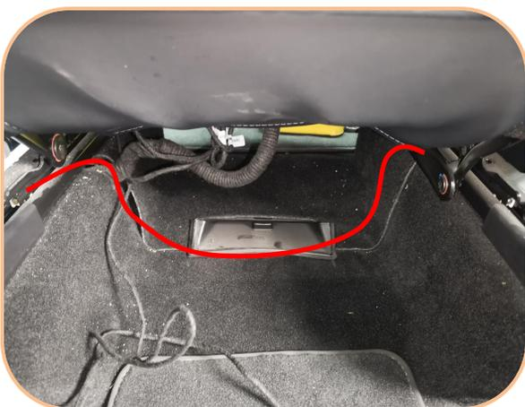
17. According to the red line, route harness (**plug ③**) from the bottom of the seat to the right side of the front right seat
