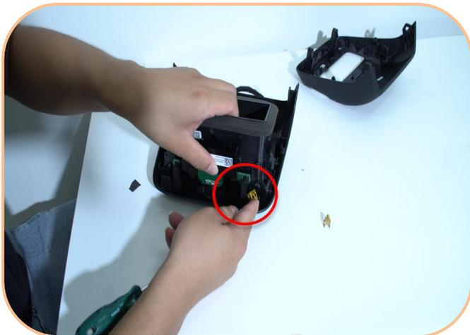
11. Install the clips onto the screen panel
