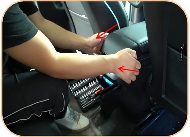
2. Pry the back of the central armrest saddle in the direction of the arrow
