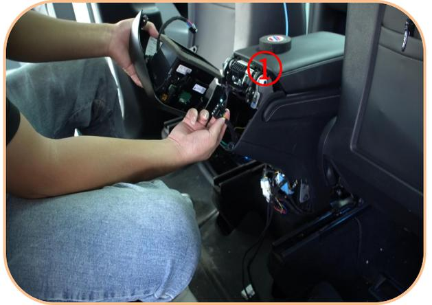
14. Connect the **plug ①** into the screen, and then connect the A/C outlet module plug
