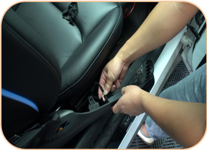
21. Unplug the seat button plug and connect the **plug ③**
