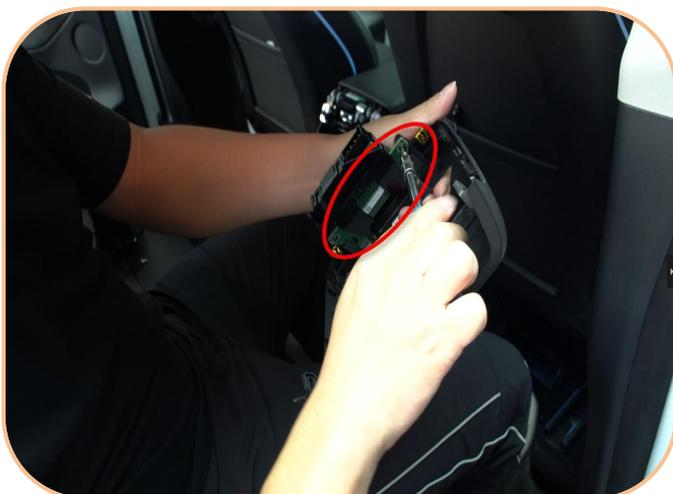
5. Unscrew the A/C outlet module screws
