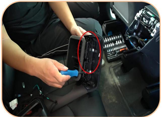
4. Unscrew the A/C outlet screw and take out the air conditioner outlet
