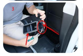
3. As shown in the picture, remove the two fixing screws of the air outlet, and then use a slotted screwdriver or pry bar to pry off the clips of the air outlet along the left and right sides; then pull out the air outlet cover, remove the two screws to take out the charging board
