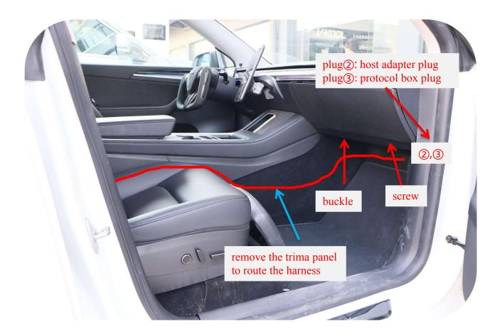
6. As shown by the arrow in the picture, route the along the armrest box: remove the inner trim panel of the armrest box, and then remove the co driver's footwell trim panel, unscrew the right screw and the left buckle.
