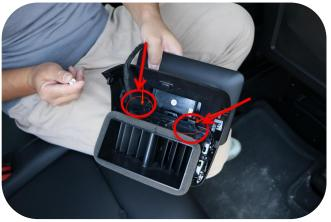
4. Fix the wireless charging board on the interior trim panel of the rear entertainment screen; and then tighten the screws. Install the air conditioner outlet above the trim panel of screen, and then tighten the screws.
