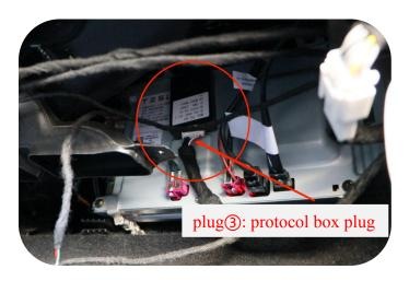
8. Connect the plug into the protocol box, paste the protocol box above the original vehicle's host and fix it,. Finally restore the trim panel.
