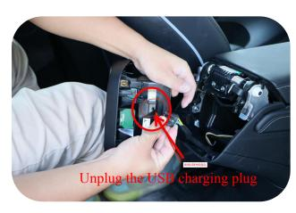
2. Unplug the USB charging plug according to the arrow in the picture
