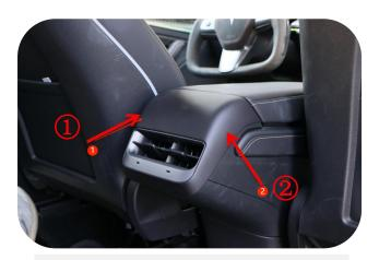
1. First, Remove the rear exhaust outlet trim panel; pull out with both hands according to the arrow
