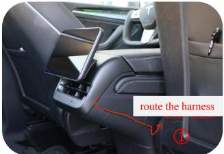
5. Connect the **power cable** ① of the screen with the **extension cable** ①, then wrap the plug with tape, and buckle the screen into the armrest box position by hand; Connect the USB charging plug to the wireless charging board, and then route the extension cable along the marking position of the armrest box to the original host position above the passenger's footwell
