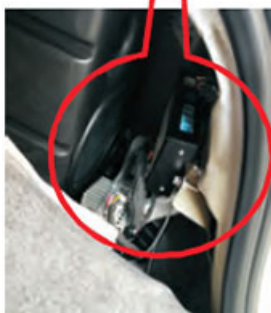
Put control box behind the right side interior lining of the trunk
