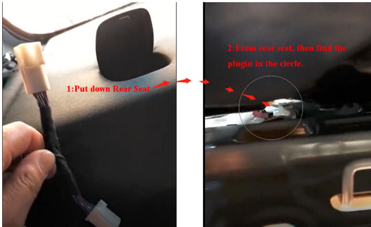
16. Tailgate signal plug location
