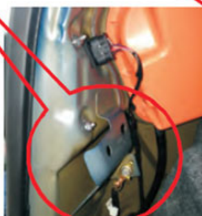
GND screw location under the tail light
