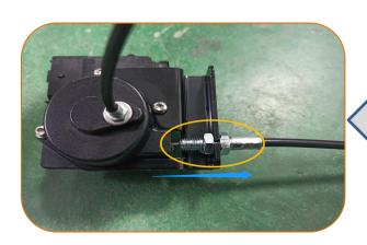
10.2 installation of suction lock If step 10-1 cannot be adjusted, adjust the screw at the lock motor and rotate it to the blue arrow. After plug in the control box and buzzer, the control box plug should be faced down, and then find a suitable position and fix it with a tie (to avoid water ingress)
