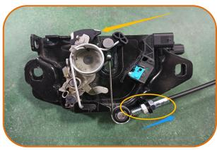
10-1. Try to hook the original spring back to the original position, check the tightness of the suction lock cable and adjust it (please do not pull the emergency cable); Adjust the screw in the direction of the blue arrow until the lock block can be fully unlocked.
