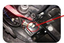
Motor adapter plug (position: next to the left headlamp of the frunk
