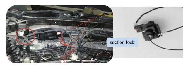
The electric suction lock must be pasted under the lock block of the original vehicle (behind the front bumper) and fixed with cable tie to prevent water from entering. The emergency cable shall be routed to the front trailer port of the original vehicle
