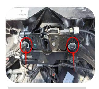
7. Unscrew two screws and remove the lock block of the original vehicle
