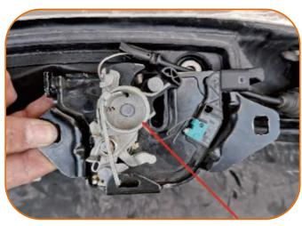
8.Remove the spring Remove the original lock block spring
