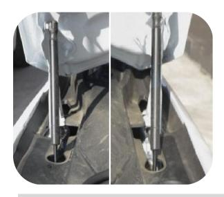
5.Remove the original hood strut, lift up the steel sheet at the back of the ball joint with a straight tool, and remove the strut. (same operation method on the left and right)
