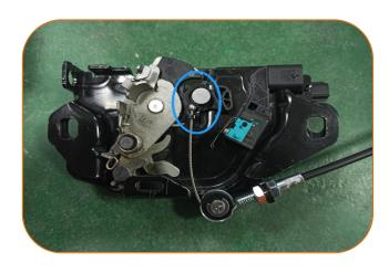
9.Install the electric suction lock Hang the small bracket on the lock hook (hanging on the spring position)
