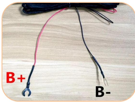
2. Thread both 12V(B+) and negative pole(B-) of power wires through the hole from the side of the rubber; the black wire (B-) connec to the orginal vehicle ground wire(negative pole)
