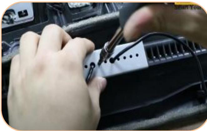
14. Pass the wiring harness through the grey fixing plate in sequence and fix the grey plate with screws
