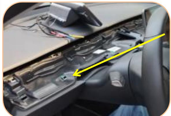
10. Remove the entire central control panel (The indicated line as shown in the picture is for wiring)
