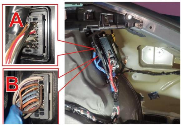
11: Install the grey connectors of the footsensor in between Plug B
