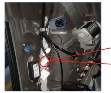
9: Install the white connectors of the footsensor in between this plug
