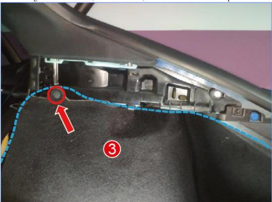
4: On the right side of the tail box, as shown below, remove the fourth interior panels
