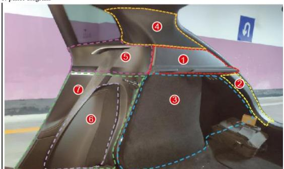
2: Put the rear seat down first, and on the rear side of the tail box, remove the first and second trim panels according to the following figure.
