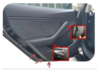
7. Remove the two screws on the front door interior trim panel and then remove the interior trim panel. There are many buckles in the interior trim panel which need pull it outward with a prying tool in the direction of the arrow
