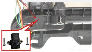
14. Install the sensor and screw onto the auto door handle (The front left, front right and rear left, rear right should correspond, Do not mixe and match)
