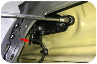
12.Unplug the sensor plug on the original outer door handle, remove the three fixing nuts, and take out the original outer door handle
