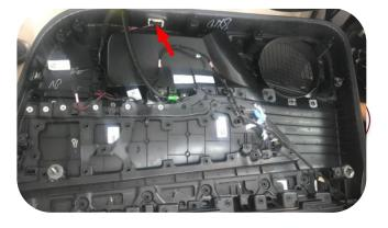
3.Disconnect the emergency wire harness from the interior trim panel and pull it off (pull out the floor lamp first, and the glass will automatically stop at the position of the removable fixing screw)
