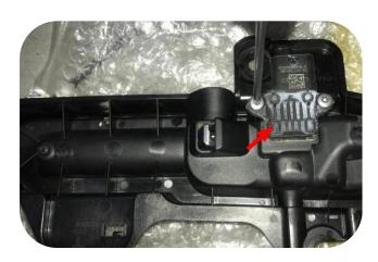
13.Unscrew the two screws and remove the sensor block (The front left, front right and rear left, rear right should correspond, Do not mix and match)
