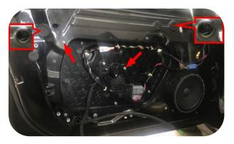
4.Remove all screws on the door inner panel, pull out the fixing clips on the wire harness and the plugs of the wire harness, then remove the door inner panel; Remove the soft rubber cover to expose the head of the glass fixing screw
