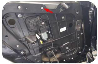
10.Then remove the #8 screw around the door inner panel and then take out the inner panel
