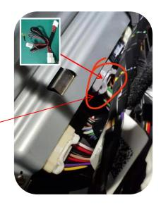
18. The main host of the original vehicle is above the upper cover plate of the front passenger side's footwell.(This plug is for Intel version, AMD version does not need to plug this plug)
