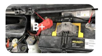
20.Thread the red wire to the frunk and connect to the small battery 12V power; Connect the black wire to the negative grounding of the original vehicle
