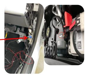
18. Thread the red wire to the frunk and connect to the small battery 12V power; Connect the black wire to the negative grounding of the original vehicle
