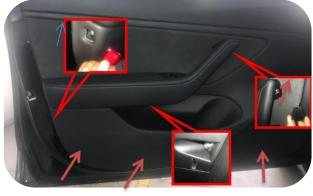
2.Remove the three screws on the front door interior trim panel and then remove the interior trim panel. There are many buckles in the interior trim panel which need pull it outward with a prying tool in the direction of the arrow
