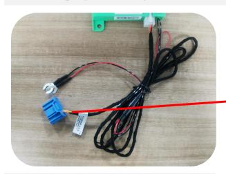
17. For AMD version: The blue plug connect to the plug under the A-pillar of the front right seat, the red is the 12V power supply, and the black is the negative pole.
