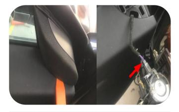
1.First raise the front door glass to the highest position, and remove the speaker on the front door, and then pull out the plug on the speaker
