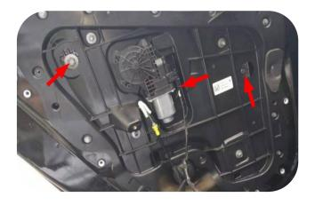
9.Unplug the window regulator motor and remove the emergency door opening pull cable
