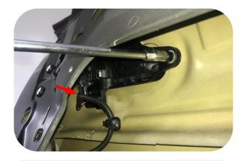
6.Unplug the sensor plug on the original outer door handle; remove the three fixing nuts, and take out the original outer door handle
