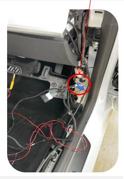
19. The blue plug is under the A-pillar of the front right seat (This plug is for AMD version, Intel version does not need to plug this plug)
