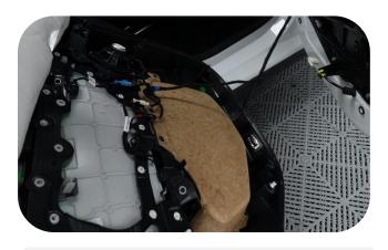
8.Adjust the upper and lower position of the glass until the fixing screw is exposed in the removal hole, and then pull out other harness plugs on the interior trim panel to separate the harness from the interior trim panel
