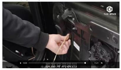
67.The cable is threaded into the car and connected to the main cable
