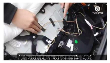
69. Remove the storage compartment light to replace the ambient light and install it back
