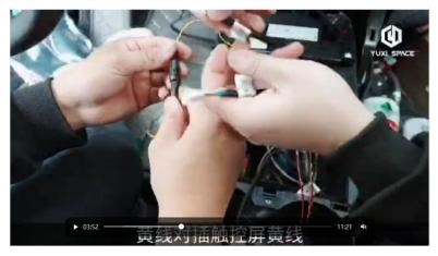
20.Plug the signal cables of both sides in the touch screen signal cables
