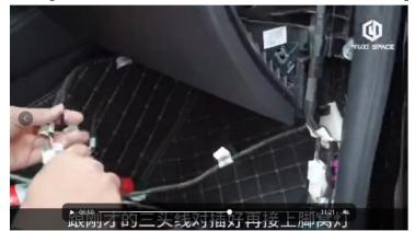
43. Arrange the wire harness and restore the cover plate
