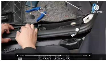
45.Remove the front door trim panel in preparation for routing
