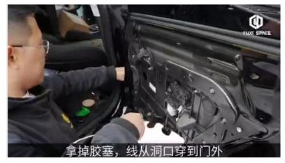
66.Rubber plug through the hole to install back
