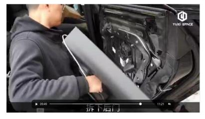
65.Remove the rubber plug, route the cable from hole to the door
