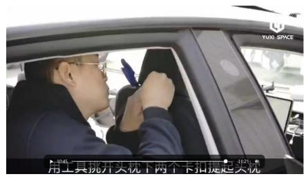
73.Remove the back of the seat to wiring
