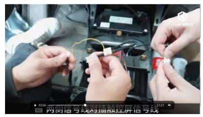
21.Plug the cable of the touch screen and arrange the cable in the bottom of the cup holder
