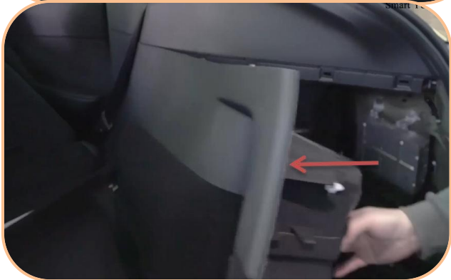
3. Pry off the trim panel cover on the right (the same operation on the left)
