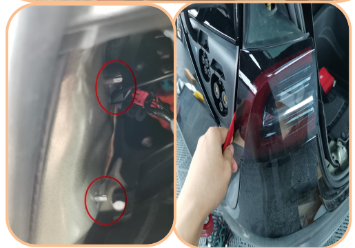
4. Pry off the rear tail light cover, unscrew two nuts on the interior trim panel, and then remove the tail light (the same operation on the left)
