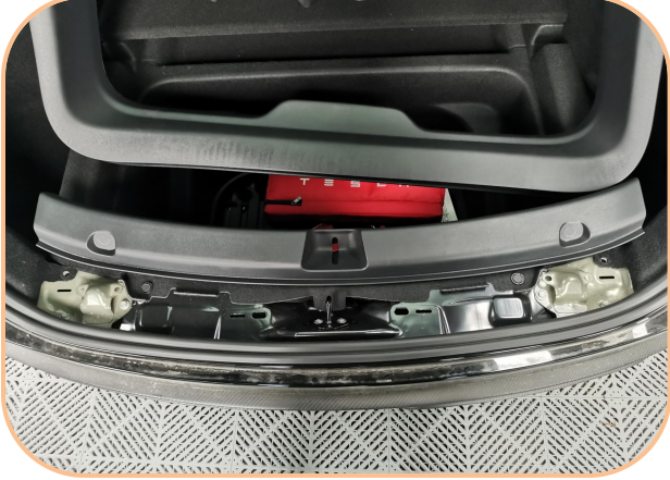
1. First remove the trunk interior trim pad
