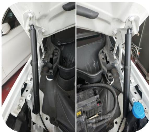
6. Remove the original strut ball joint; **Install the new bracket (left and right are the same) See page 4 for details.** After installation, manually shake the strut ball joint to check whether the ball joint is firmly installed
