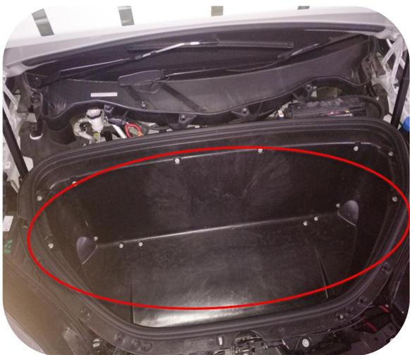
3. Remove the Frunk spare box (remove the original vehicle screws first)
