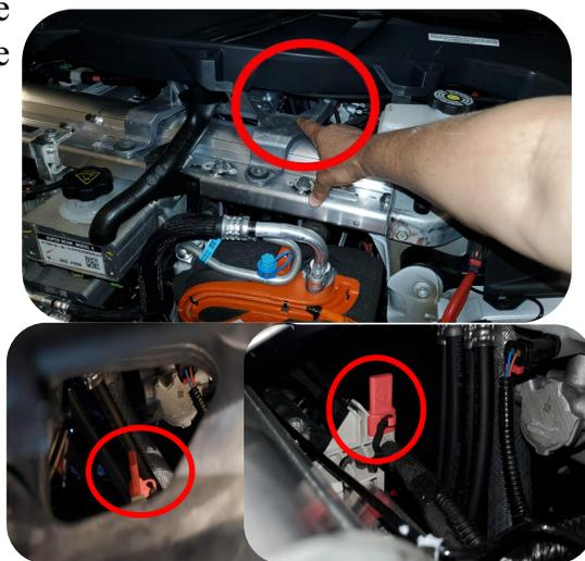
Connect the negative pole to the negative grounding position of the original vehicle
