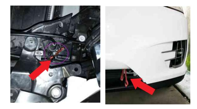
Take the emergency pull cord of the actuator of the electric suction lock to the vicinity of the through - hole at the bottom of the right side of the figure, and fasten it with the cable tie to keep the tension pull ring in the loose reset status.
