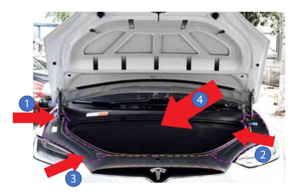
Remove the remaining trims in order. First remove the two side panels, then remove front trim, after removing the trim, remove the 2 lamps in the frunk, and take out the flannel trim.
