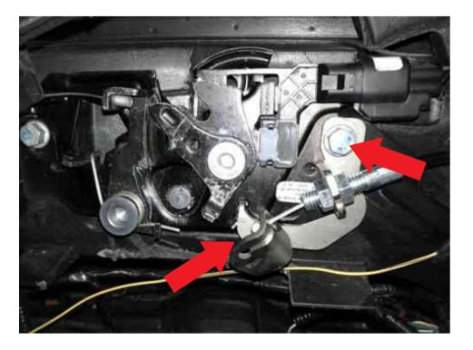
Mount the bracket of the electric suction lock to the original car lock hook hole, install the bracket to the screw on the right side as shown.
