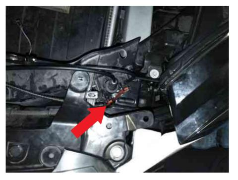
The electric suction lock must be installed under the original car lock block (behind the front bumper) and secured with a tie to prevent water ingress.
