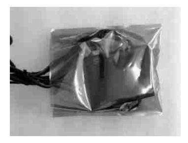
Note: After all the plugs of the control box are plugged in, Put the control box and buzzer in our anti - static bag, tie all the harness with a tie, and tie the mouth of the anti - static bag.
