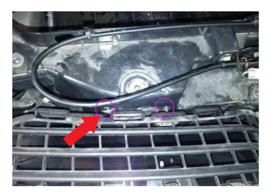
After removing the two panels with the logo, you can see the screws on the back of the front cover button. Remove these 2 screws.
