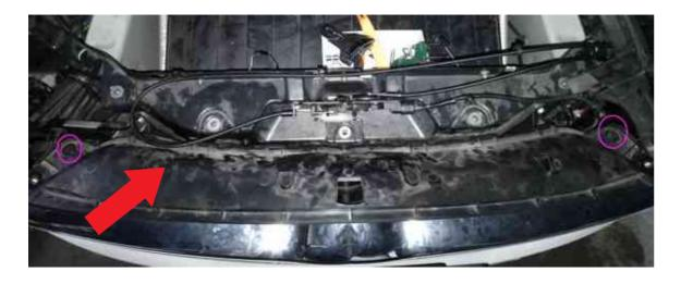
Remove the buckle of the first panel and then remove the second panel.
