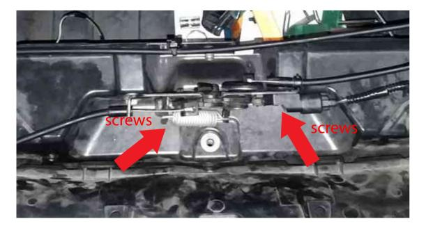
Mark the lock block installation position first, then remove the original car lock block plug and the pull cord. Use a wrench to loosen the lock block screws and take out the lock block.
