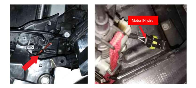
Motor plug position is here as shown, find the Motor plug, connect our yellow motor IN wire to the white wire of the motor plug.
