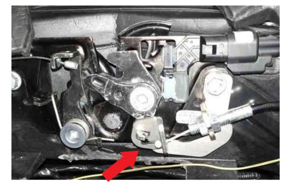
Install the metal bracket with the pull wire as shown. (position of the spring hook).
