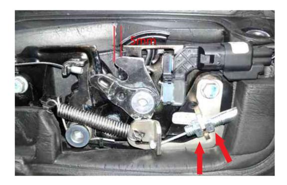
After finish the installation, please try to make the electric suction work several times. If the lock hook does not hang the door lock ring and fails to suck the door down or the door lock ring is closed and hits the lock hook. Please adjust the two nuts shown in the figure, make the hook move about 5mm left from central, to make the latch can go into the hook easily when closing.
