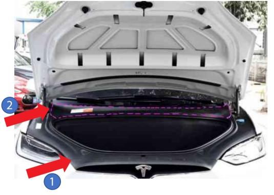
Open the trunk and take the trunk waterproof seal out first. Next, remove the panel as shown. 2. Removal of the front trim panel
