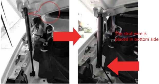
Use a small screwdriver to lift the steel spring on the back of the ball and remove the strut. Replace it to our electric struts. (The figure shows is the installation method on the right side)
