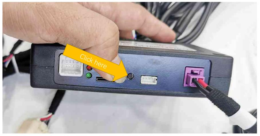
Press and hold for 3 seconds, then press for another second to increase the strength of the electric tailgate (a total of 5 intensity adjustment)
