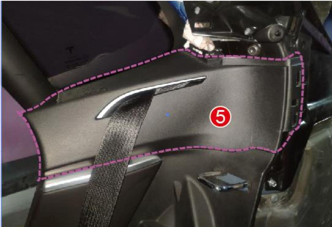
6: After removing the fifth interior panel, as shown in the figure, remove the two buckles, and then remove the sixth and seventh interior panels
