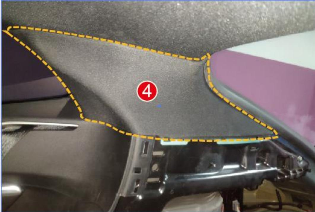
5: On the right side of the rear seat, as shown in the figure below, remove the fifth interior panels
