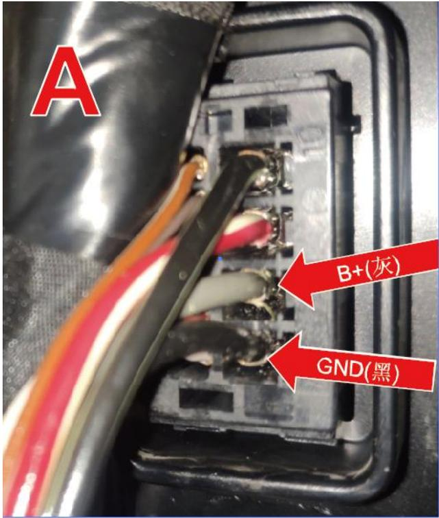
12: Plug A, connect the red wire (+12V) to the constant powered 12V, and connect the back (GND) wire to the ground.
