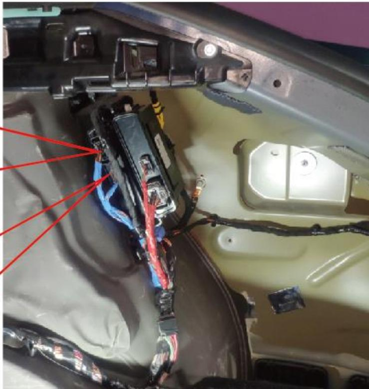
11: Install the grey connectors of the footsensor in between Plug B
