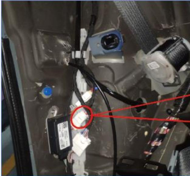
9: Install the white connectors of the footsensor in between this plug
