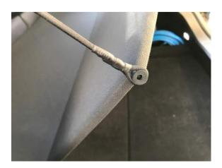
Now connect the elastic wire to the screw and grommet, and you are finished. If you need to remove the parcel shelf, we recommend releasing the wire from the screw.
