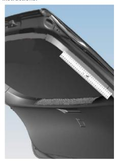
Measure 27 cm's from the gap between the lower part of the rear hatch liner and the side part. Mark the position where the screw should be inserted.
