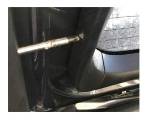
Now insert the pin through the rubber grommet as seen in the picture and push it into the parcelshelf at an angle of approximate 45 degrees forward. Be sure that the pin keeps centred in the parcel shelf, so it doesn't come out in the bottom or top.
