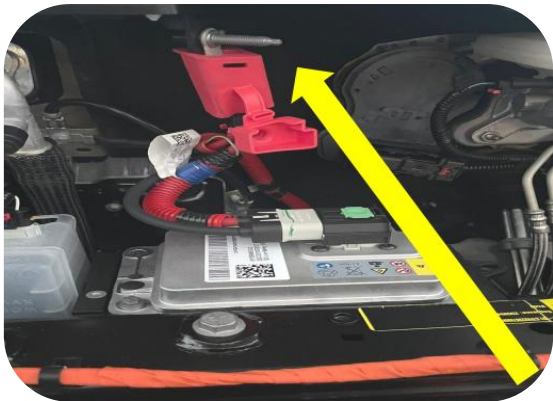
Model Y : Positive pole power position
