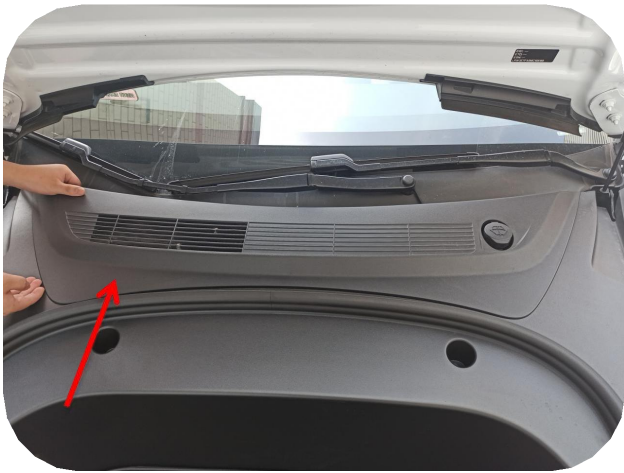
1. Remove the conditioning filter element cover and take out the cover
