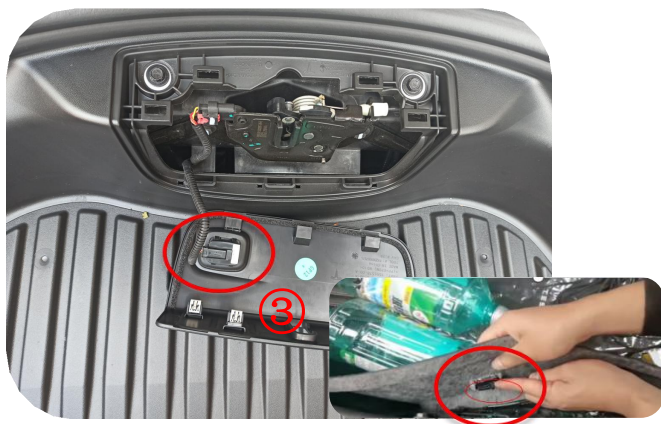
Model X AMD Version: Positive pole power position
