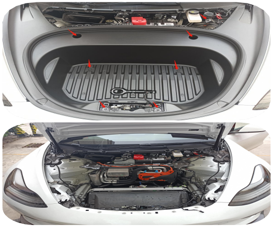
2. Remove the screws as shown by the arrow, Remove the front spare box and connect the harness
