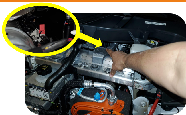
Model X AMD Version: Positive pole power position
