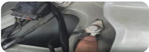
Model 3 AMD Version positive pole fixing screw
