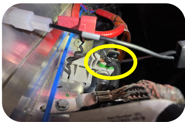
Model S AMD Version: Positive pole power position
