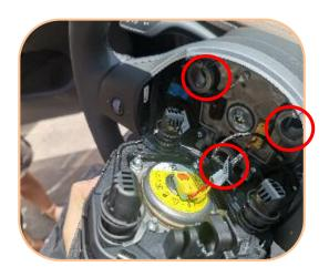
11. Finally, insert the airbag plug, and insert the airbag into the spring bayonet.
