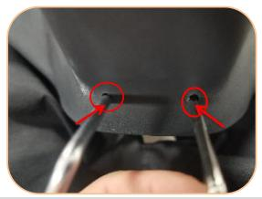
3. There is a hole on the left and right sides of the steering wheel. Insert and Jack the airbag spring with a flat head screwdriver respectively.
