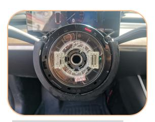
9. Do not turn the hairspring after pulling out the steering wheel.
