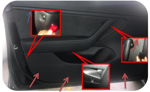
2. Remove the three screws on the front door interior trim panel and then remove the interior trim panel. There are many buckles in the interior trim panel which need pull it outward with a prying tool in the direction of the arrow
