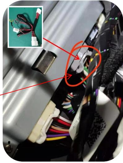
17. **For Intel version:** The blue plug connect to the plug under the A-pillar of the front right seat, The white plug is connected to the plug of the host of the original vehicle; the red is the 12V power supply, and the black is the negative pole. (This step is for Intel Version, AMD Version pls refer to Page 4)
