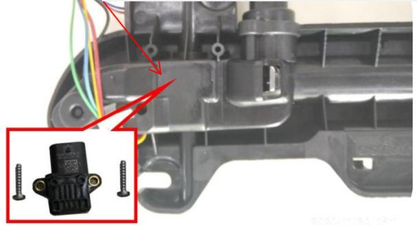
14. Install the sensor and screw onto the auto door handle (The front left, front right and rear left, rear right should correspond, Do not mix and match)
