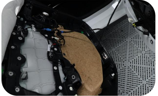
7. Remove the two screws on the front door interior trim panel and then remove the interior trim panel. There are many buckles in the interior trim panel which need pull it outward with a prying tool in the direction of the arrow
