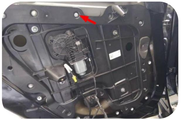
9. Unplug the window regulator motor and remove the emergency door opening pull cable
