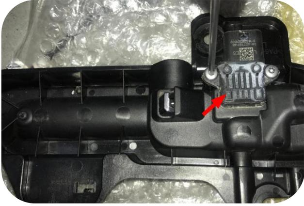
13. Unscrew the two screws and remove the sensor block (The front left, front right and rear left, rear right should correspond, Do not mix and match)
