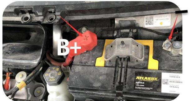
20. Thread the red wire to the frunk and connect to the small battery 12V power; Connect the black wire to the negative grounding of the original vehicle
