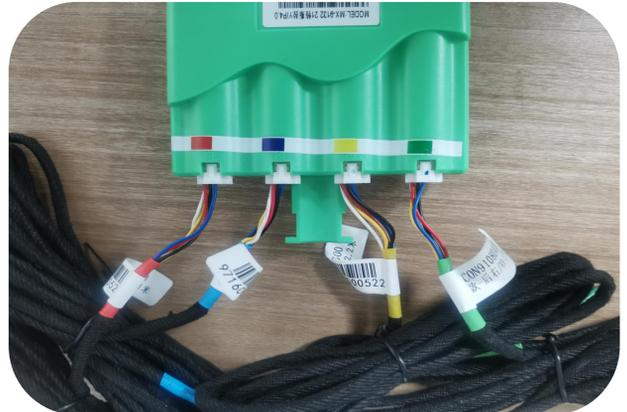
16. The wiring of the control box shall be inserted according to the corresponding color, and the control box shall be fixed on the front right footwell cover plate (see the wiring diagram on page 1 for details)
