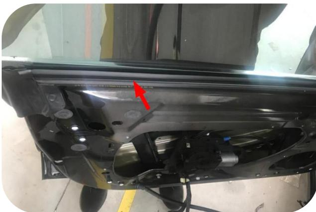
5. Remove the fixing screws of the glass; remove the glass adhesive strip and then take off the glass
