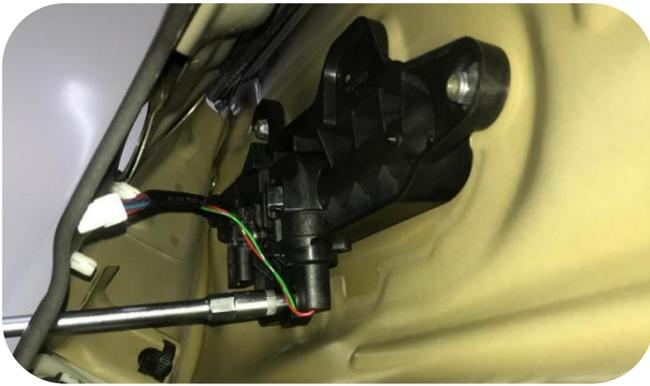
15. Install the Auto door handle onto the corresponding door and tighten the nuts; Before fastening the nuts, the gap between the handle and the door can be properly adjusted to ensure that the gap is uniform and beautiful, and then insert the sensor plug on the original vehicle
