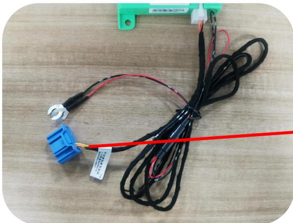
17. **For AMD version:** The blue plug connect to the plug under the A-pillar of the front right seat, the red is the 12V power supply, and the black is the negative pole. (This step is for AMD Version, Intel Version pls refer to Page 5)
