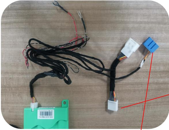
17. **For Intel version:** The blue plug connect to the plug under the A-pillar of the front right seat, The white plug is connected to the plug of the host of the original vehicle; the red is the 12V power supply, and the black is the negative pole. (This step is for Intel Version, AMD Version pls refer to Page 4)
