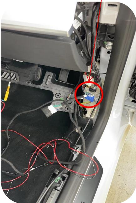
19. The blue plug is under the A-pillar of the front right seat (This plug is for AMD version, Intel version does not need to plug this plug)
