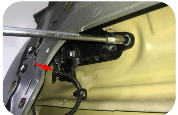
6. Unplug the sensor plug on the original outer door handle; remove the three fixing nuts, and take out the original outer door handle
