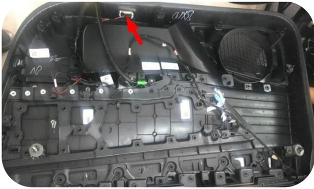
3. Disconnect the emergency wire harness from the interior trim panel and pull it off (pull out the floor lamp first, and the glass will automatically stop at the position of the removable fixing screw)
