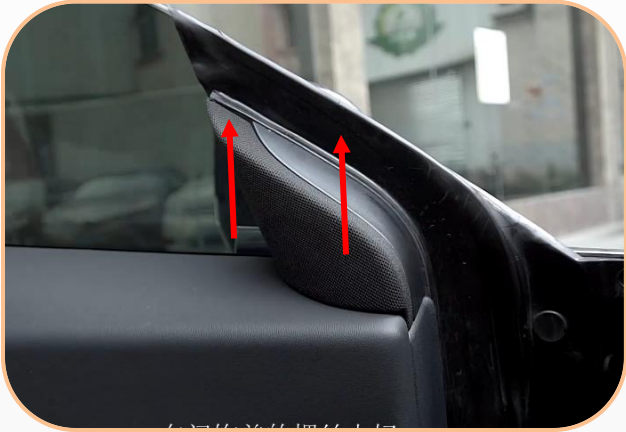
2.Lift the triangular tweeter up and unplug the tweeter plug
