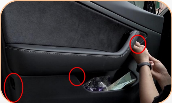
3.There are 3 screws on the door panel handle,and then pry open the door panel with the prying tool
