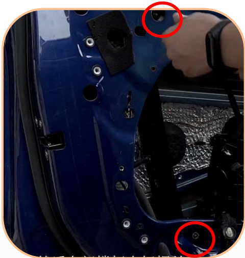
17.Screw back the two screws of the window regulator
