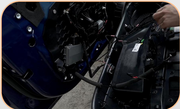
24.Connect the pull cable of the door panel and the plug
