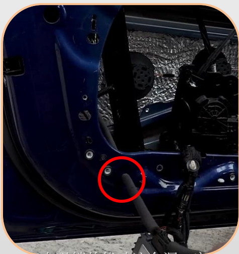
16.Take the electric suction lock pull cable out of the original hole
