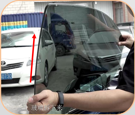
8.Lift the window glass up carefully
