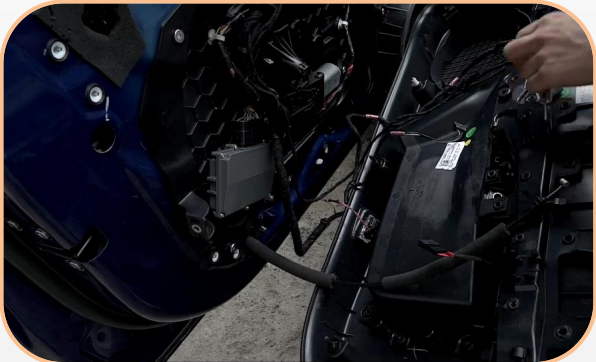
4.After prying the door panel, remove the plug connecting the door panel
