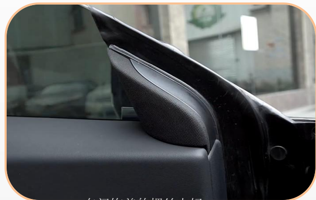
27.Install back the triangle tweeter and complete the installation
