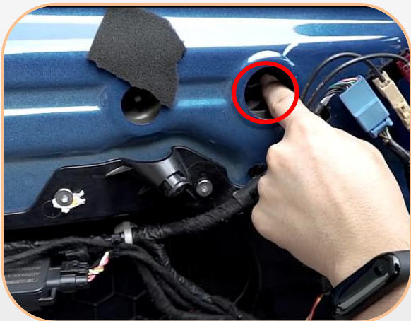
21.Align the screw holes of the glass and the lifting frame, and screw the original vehicle screws (with two holes)
