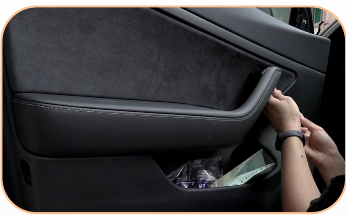
26.Screw back the three screws of the door panel
