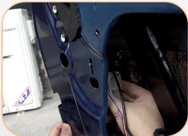
14.Replace with new electric suction lock and plug in the plug of the original car
