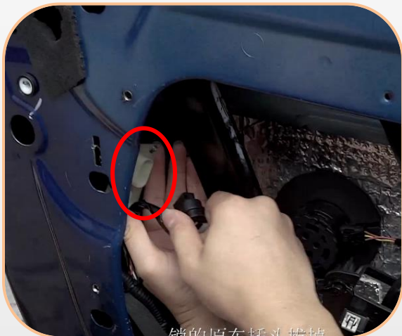
13.Unplug the electric suction plug and take down the electric suction lock of the original vehicle
