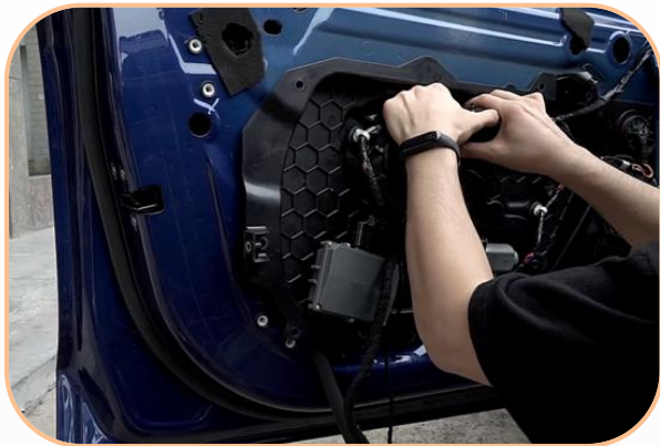
9.Unscrew the screws of the inner plate and disassemble the original trunking
