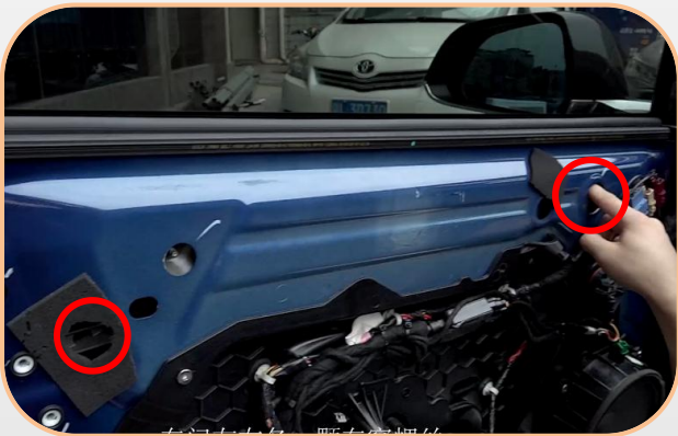
6.Unscrew the two screws of the window
