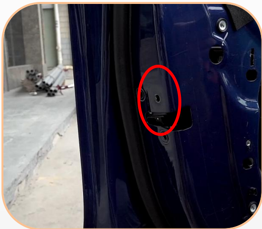
11.Unscrew the 3 screws of the original electric suction lock
