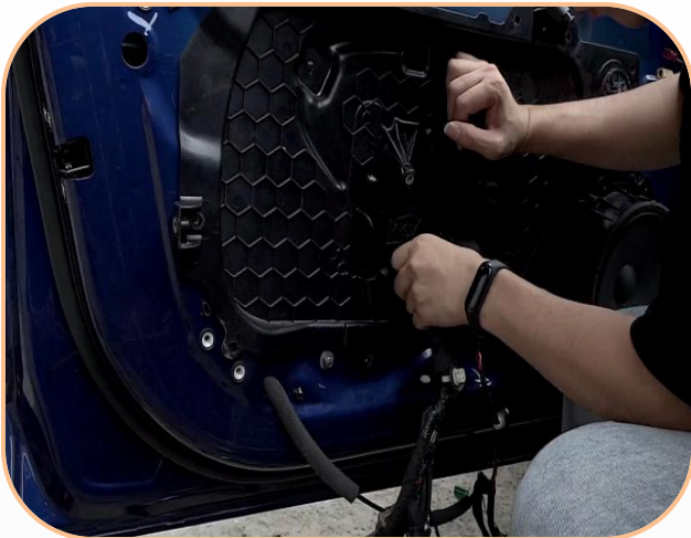
18.Install back the inner plate and screw back the screws
