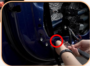
12.Unscrew the two screws of the window regulator
