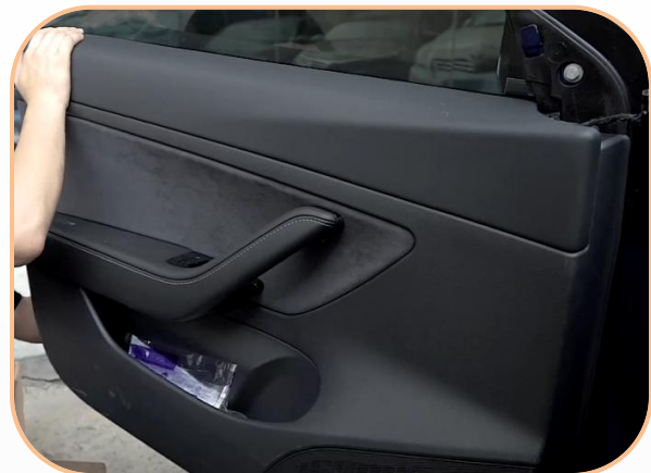
25.Align the door panel and install the buckle
