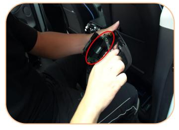
5.Unscrew the A/C outlet module screws
