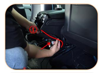
13. Pull harness with plug (1) to the upper part and restore the cover plate
