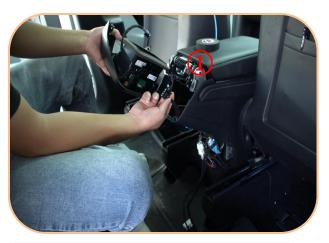
14. Connect the plug ① into the screen, and then connect the A/C outlet module plug
