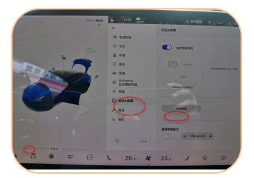
1. Turn off the vehicle power in the vehicle setting
