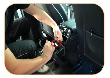
3. Pull off the A/C outlet module plug
