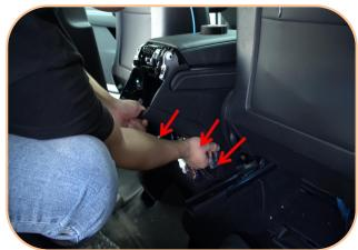
12. Pry the cover plate behind the sentral armrest saddle in the direction of the arrow
