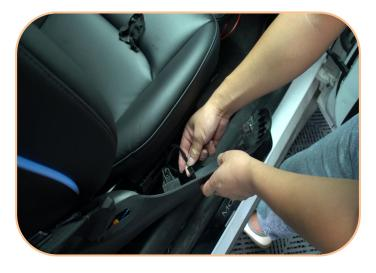
21. Unplug the seat button plug and connect the plug (3)
