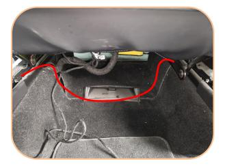
17. According to the red line, route harness (plug (3)) from the bottom of the seat to the right side of the front right seat
