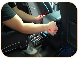
2. Pry the back of the central armrest saddle in the direction of the arrow
