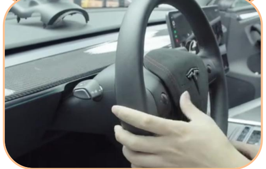
1. Slide the steering wheel to the bottom and then turn left to move the steering wheel to the the outermost position
