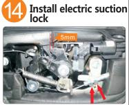
fter finish the installation, please try to make the electric uction work several times. If the lock hook does not hang be door lock ring and fails to suck the door down or the oor lock ring is closed and hits the lock hook.Please adjust le two nuts shown in the figure, make the hook move about mm left from central, to make the latch can go into the hook asily when closing.
