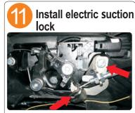
Mount the bracket hook of the electric suction lock to the original car lock hook hole, install the bracket to the screw on the right side as shown.
