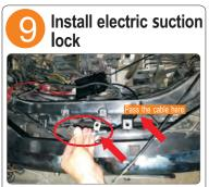
Passed the electric suction lock with the bracket part out from the bottom to another side.
