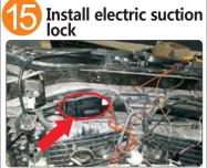
The electric suction lock must be affixed under the original car lock block (behind the front bumper) and secured with a tie to prevent water ingress.
