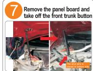
Use a screwdriver to lift the steel sheet back of the ball head and remove the support strut. Replace it to our electric struts. (The figure shows the installation process on the right side) Strut wire should be on the bottom.
