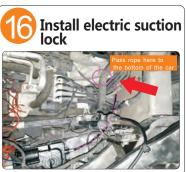
Take the emergency pull cord of the actuator of the electric suction lock to the vicinity of the through-hole at the bottom of the right side of the figure, and fasten it with the cable ite to keep the tension pull ring in the loose reset status.
