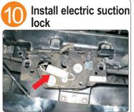
Remove the original car lock block spring.
