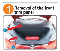
Open the trunk and take the trunk waterproof seal first. Next, remove the panel as shown.
