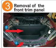
Remove the lock block trim and remove the front box flannel trim.
