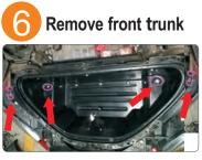
Remove the front box, four screws on the left and right sides, and two screws on the inside.
