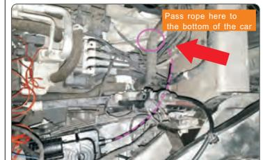
Take the emergency pull cord of the actuator of the electric suction lock to the vicinity of the through-hole at the bottom of the right side of the figure, and fasten it with the cable tie to keep the tension pull ring in the loose reset status.
