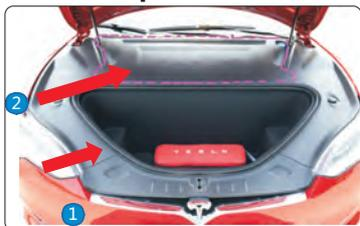
Open the trunk and take the trunk waterproof seal first. Next, remove the panel as shown.
