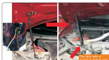
Use a screwdriver to lift the steel sheet back of the ball head and remove the support strut. Replace it to our electric struts. (The figure shows the installation process on the right side). Strut wire should be on the bottom.
