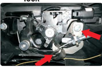
Mount the bracket hook of the electric suction lock to the original car lock hook hole, install the bracket to the screw on the right side as shown.
