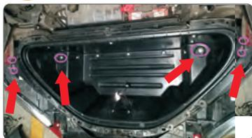
Remove the front box, four screws on the left and right sides, and two screws on the inside.
