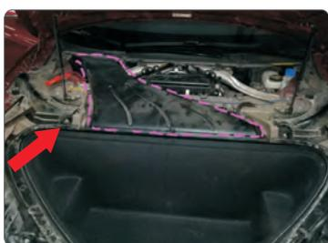
Please remove the air conditioning intake pipe and do it carefully.
