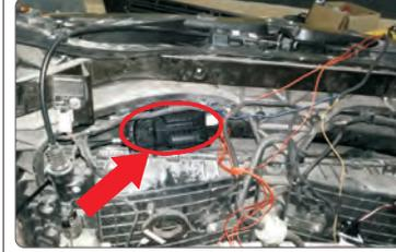
The electric suction lock must be affixed under the original car lock block (behind the front bumper) and secured with a tie to prevent water ingress.
