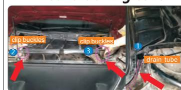
First, remove the drain tube on both sides of the air conditioner cover (remember to plug it back when restoring). The buckles on the left and right sides of the air conditioner cover can be removed after pulling the buckles (as shown)
