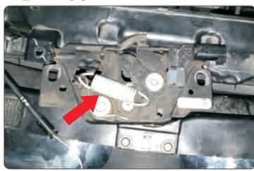
Remove the original car lock block spring.
