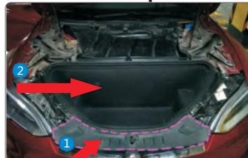
Remove the lock block trim and remove the front box flannel trim.
