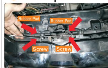
Mark the lock block installation position first, then remove the original car lock block plug and the pull rope. Use a wrench to loosen the lock block screws and remove the lock block.
