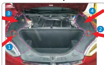
Remove the remaining trims in order, firstly remove the two side panel rubber screws, then remove 2 side trim, after removing the trim.
