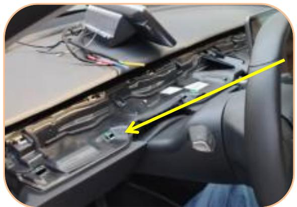
9. Then thread the wire harness to this position, as shown in the figure
