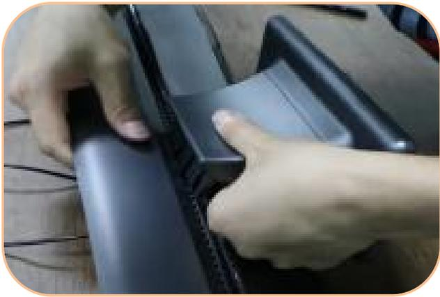
Note: The base here must be pressed to the bottom, make sure to insert the buckles in parallel when installing, if not pressed to the bottom, the screen may shake up and down after tightening the screws
