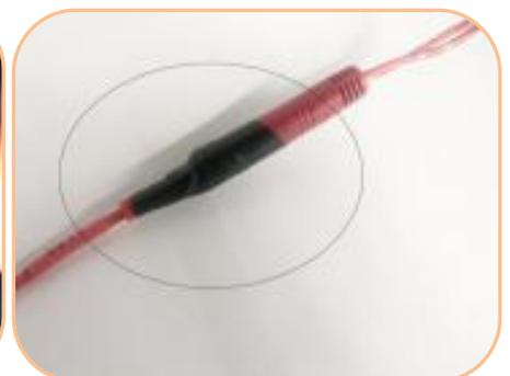
15. After fixing the plate, insert the plugs corresponding to all colors, (Note: Connect the red wire with red color; and blue wire with blue color)
