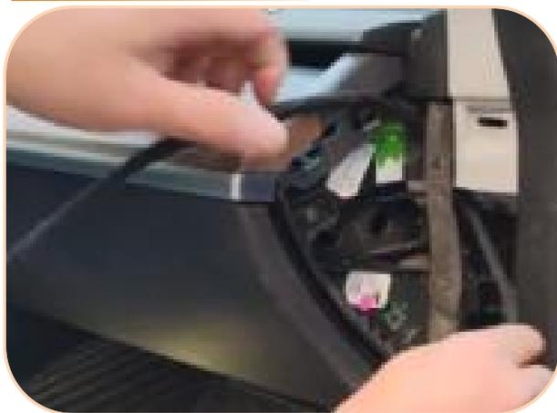
1.Remove the left and right trim panels of the central control panel
