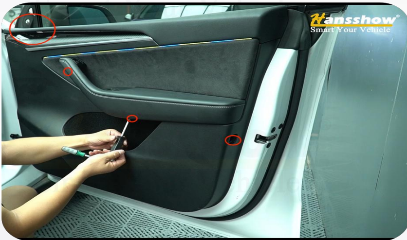
27. Secure the three screws and then install the speaker
