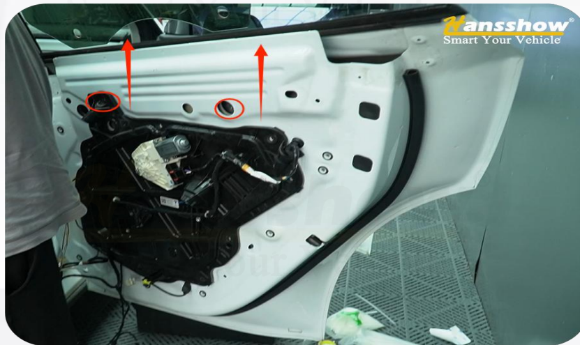
31. Loosen the two screws and remove the car window
