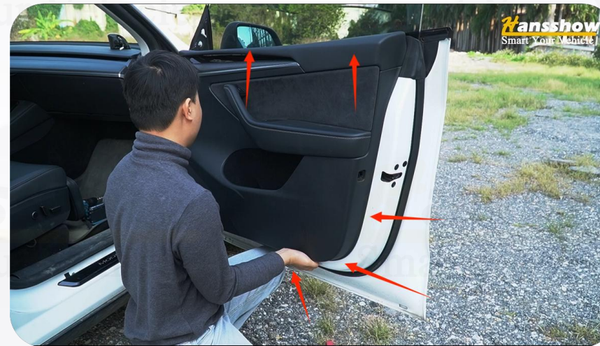
4. Use a pry bar to pry it open and then lift it upwards to remove the door trim panel
