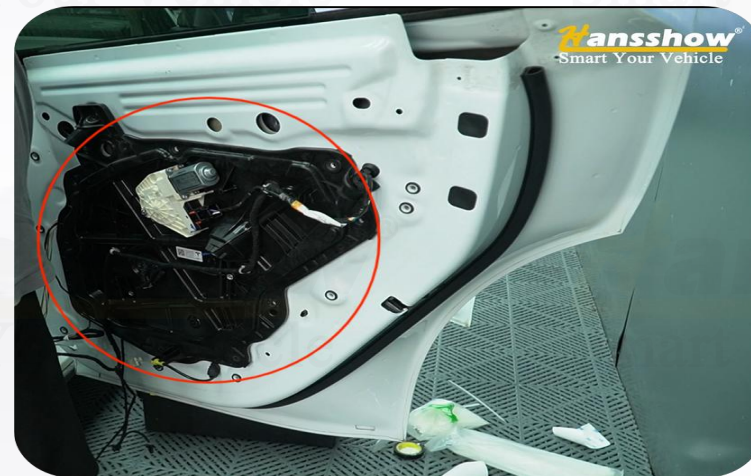
32. Loosen the screws around the inner panel
