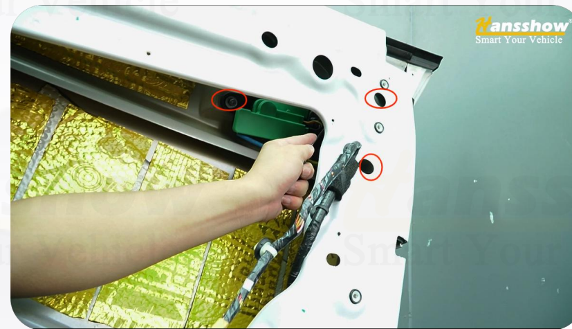
12. Loosen the screws along these three locations and unplug the door handle connector
