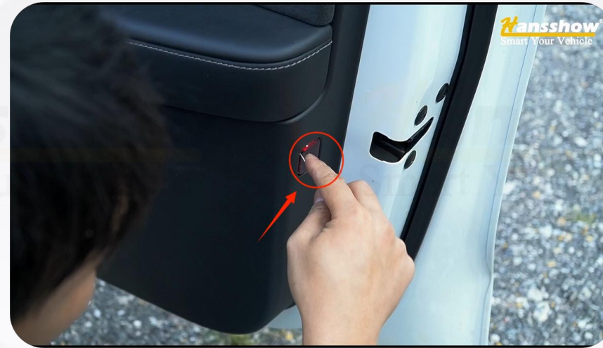
2. Pry open this and then unscrew the screw
