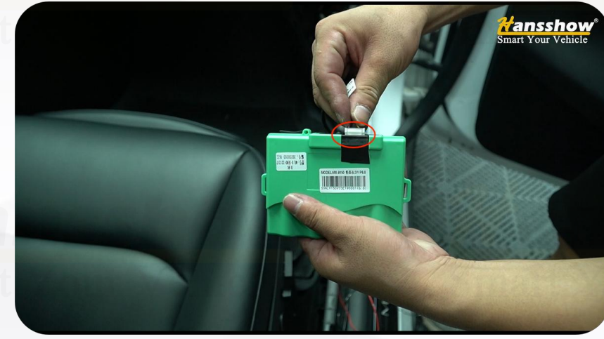
40. Plug the power cable (white plug) into the control box
