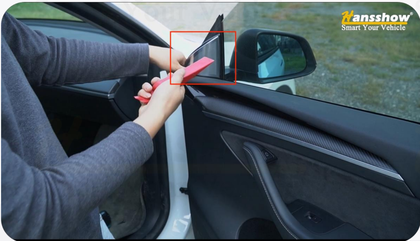
3. Pry open this speaker and then unplug the connector
