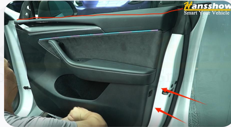
26. After installing the window sealing strip, reinstall the car door
