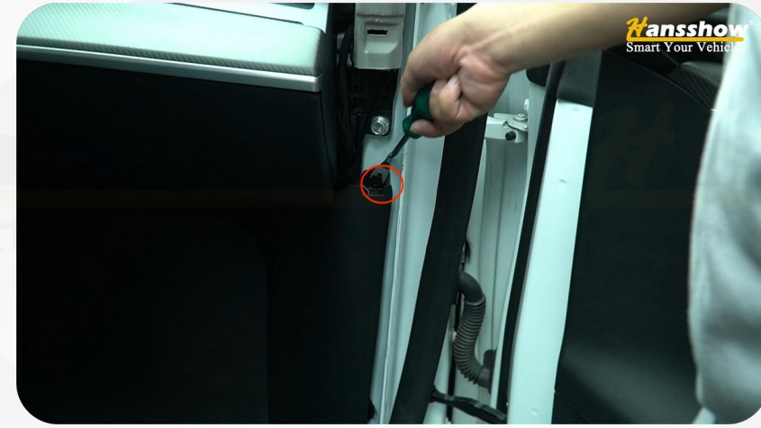
38. Pry open this clip and remove the kick plate
