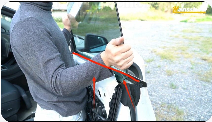
7. Remove the window sealing strip and then lift the glass upwards to extract it
